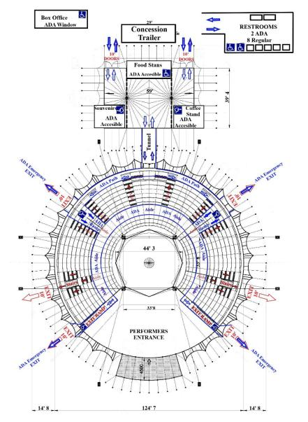
**Circus Vargas ADA ACCESSIBILITY Layout and path** Blue lines and Blue arrows are path for ADA Wheel Chairs Every seatting Section has ADA avilibility with a total of 20 avaliable ADA seating and 40 additional seats for ADA Companions. Total Maximun Seating Capacity 1032
