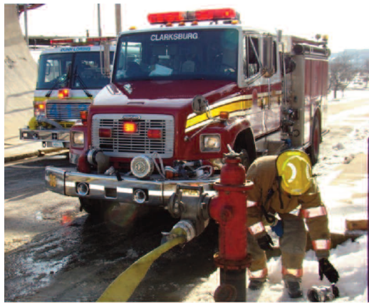
Figure 16: Connecting to the Hydrant
