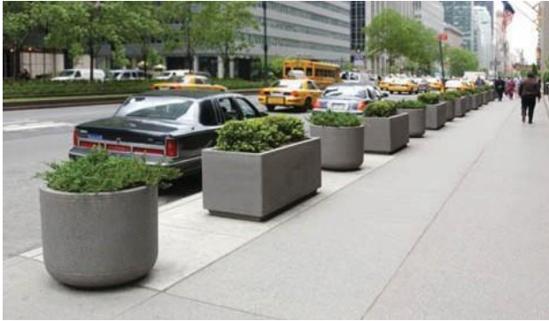
Concrete planters serve as a pedestrian buffer
