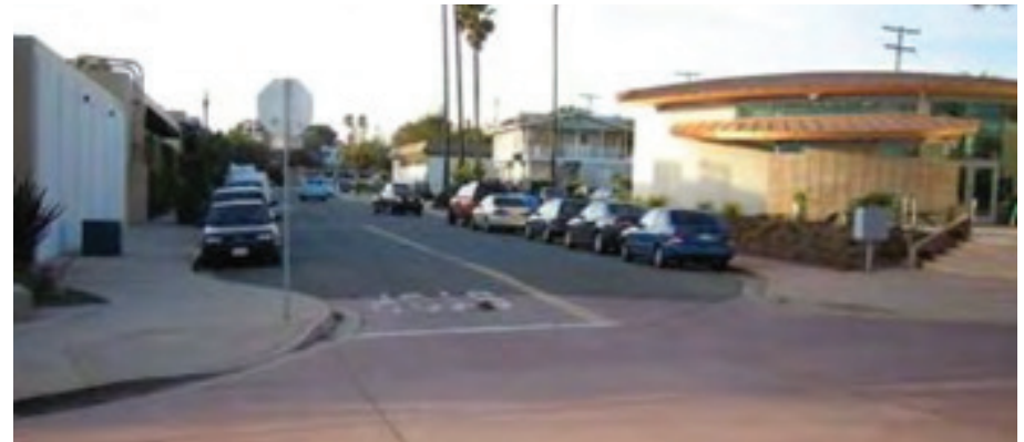
Example of a bulb-out at an intersection
