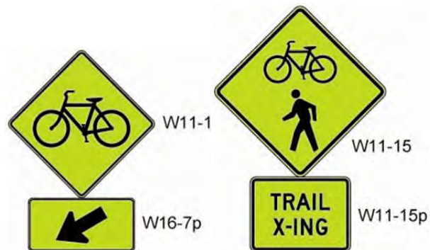
Recommended signage from FHWA-MUTCD, Figure 9B-3
