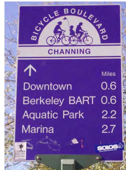
Wayfinding that includes distance and time can aid bicyclists in route finding.
