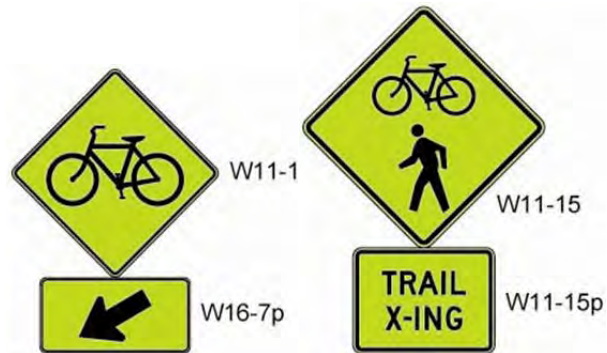
Recommended signage from FHWA-MUTCD, Figure 9B-3
