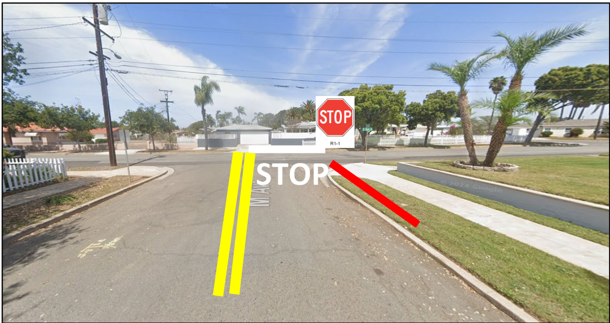
Install Stop Control sign on M Avenue and 28 th Street (looking north)
