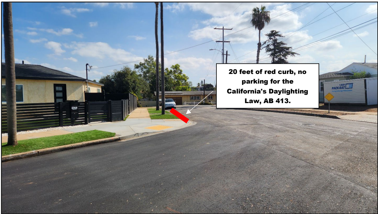
Install 20 feet of red curb “No Parking” on the north side of 28th Street, east of Virginia Drive to comply with daylighting laws (looking east)
